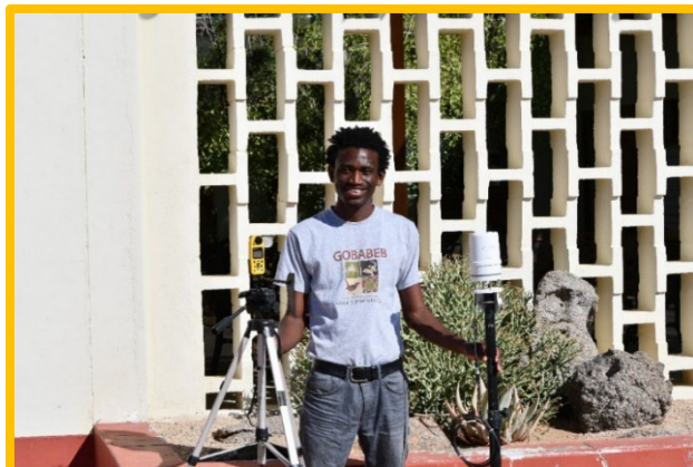
Mr Ndelimona lipinge, one of Gobabeb's Student Associates and MSc student at UCT with the two instruments to enhance work in the field. Left is the portable Kestrel 5500 weather meter and the ClimaVue sensor.
