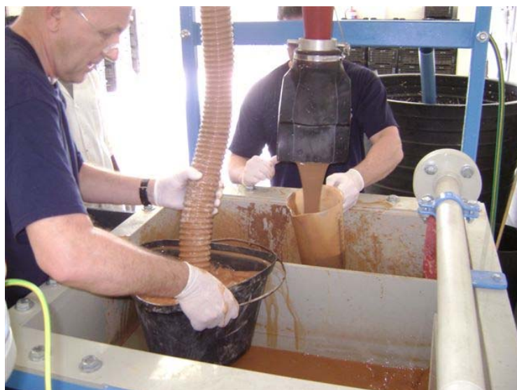
Cyclone under- and overflow being collected during operation
