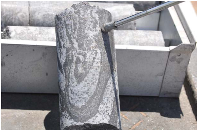
Figure 4: Shiyela PQ Core Showing Folded Magnetite Bands
