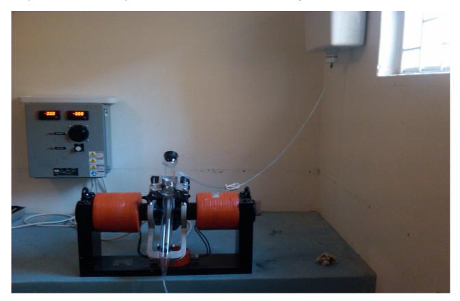
Photograph shows RUN's Davis Tube apparatus consisting of a glass tube which is agitated within an electromagnetic field. A static-head water wash is used to help remove non-magnetic material
