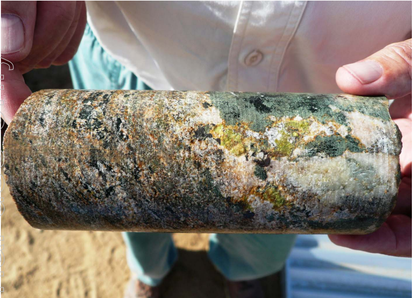
Figure 3: HQ diamond drillcore – altered granitic host rock with black magnetite, dull green skarn minerals and yellow-green secondary uranium mineralisation (uranophane and beta-uranophane).
