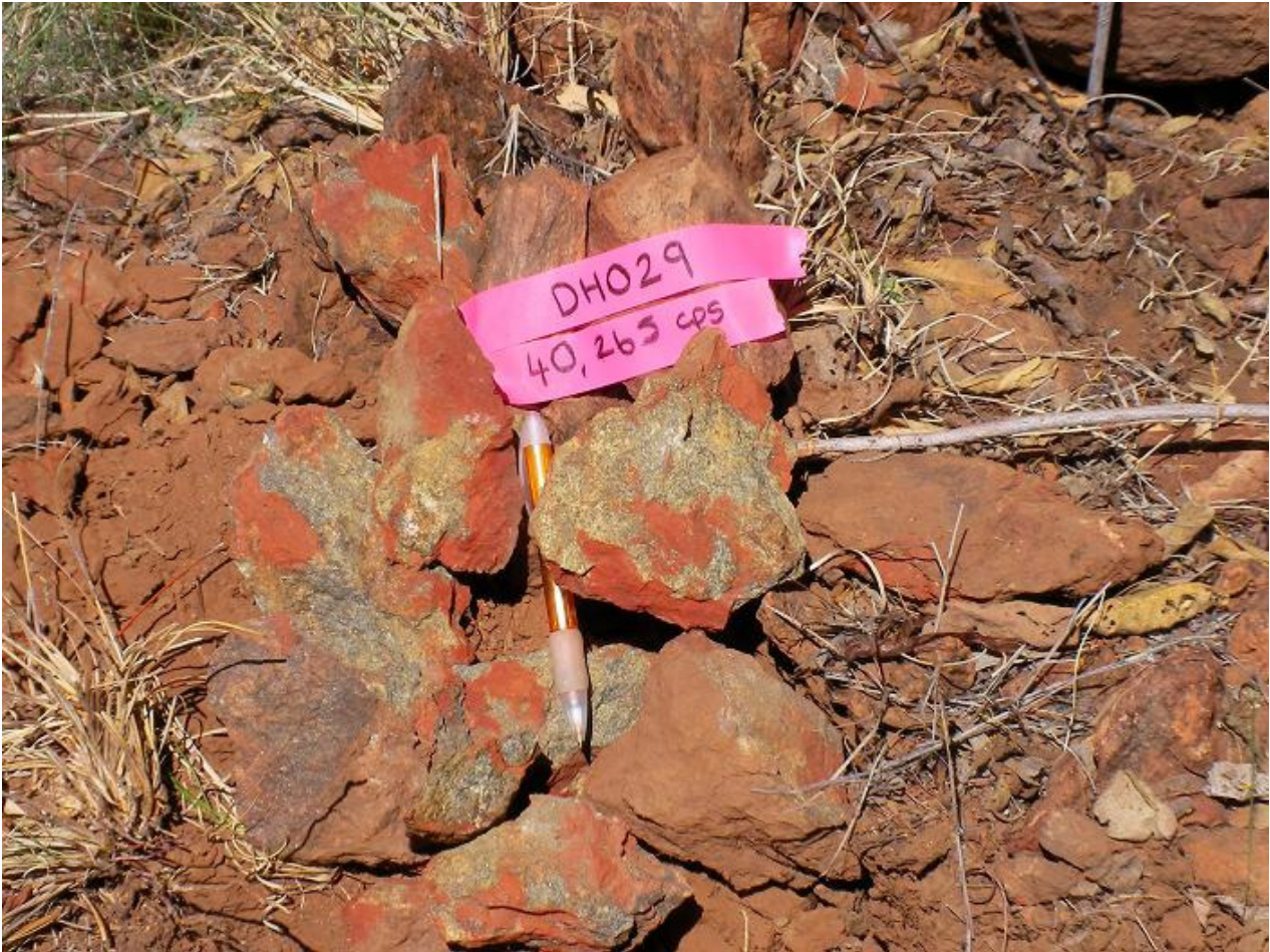
Miranda North Sample DH 029. Oxidised chlorite–haematite schist with pale yellow uranophane (?) mineralisation
