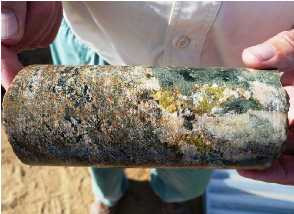
Photo of INCA HQ diamond drillcore – altered granitic host rock with black magnetite, dull green skarn minerals and yellow-green secondary uranium mineralisation (uranophane and beta-uranophane).
