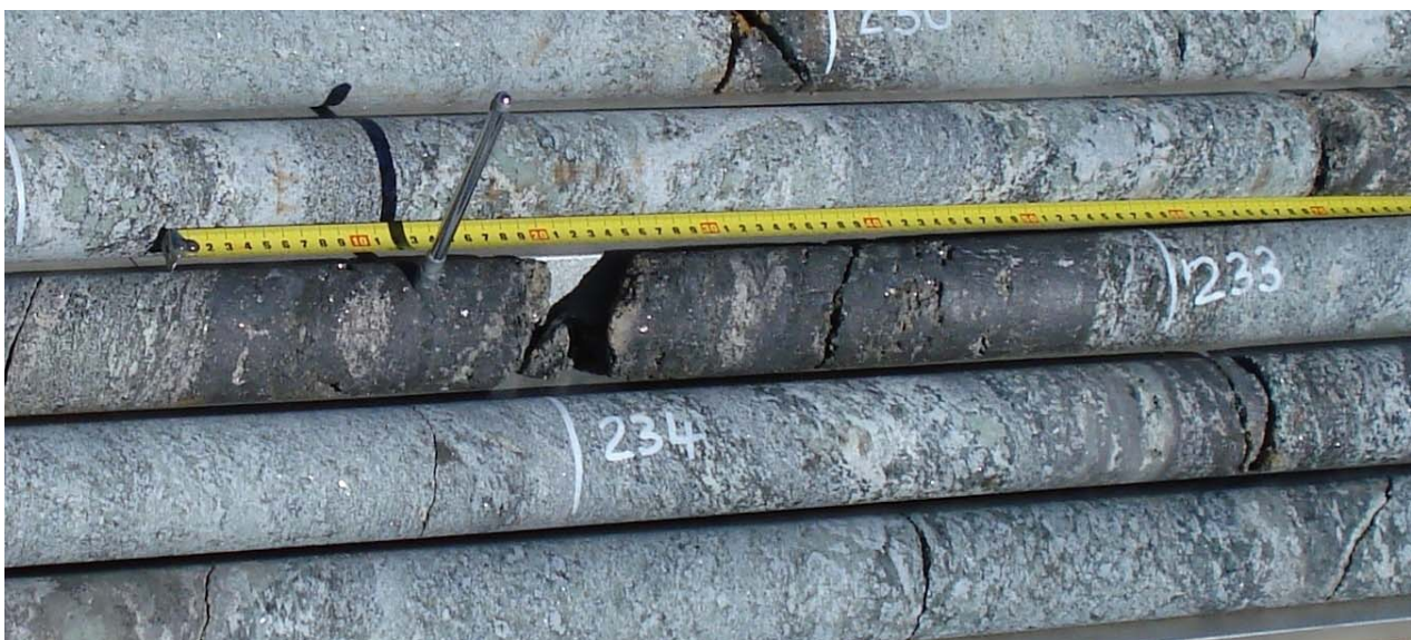
Figure 2: Diamond core from hole INCD7 showing massive highly mineralised magnetite, brecciation and alteration.
