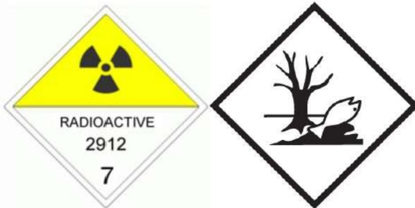
**Figure 8.3: Radioactive 7 and Environmentally Hazardous Substance (NOS) placards**
