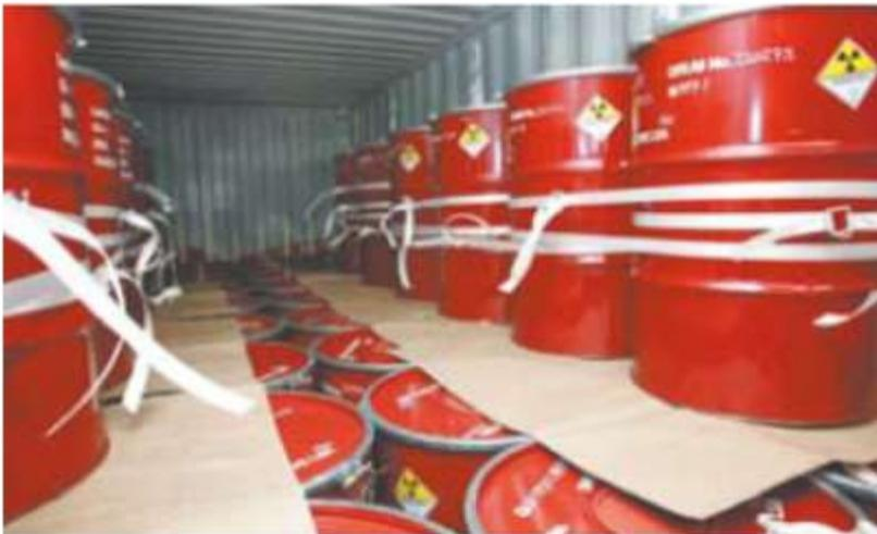
**Figure 8.1: Drums fastened and secured safely within a GP container.**
