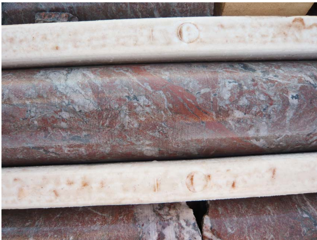
Close-up of hematite alteration – brecciation – Hole QGDC001
