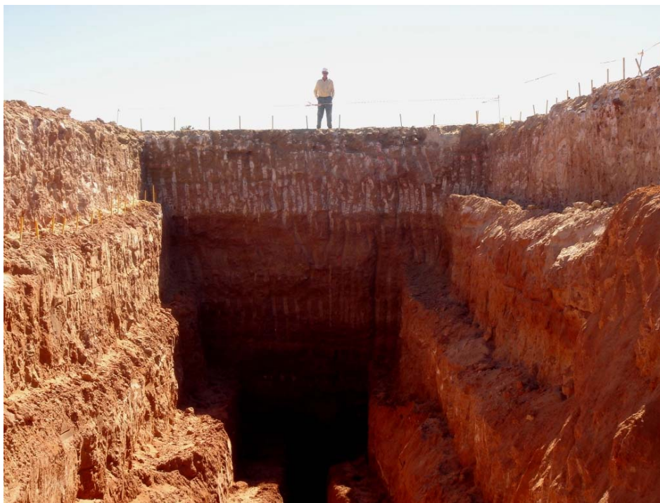
Tubas: Final trench profile showing upper gypsum layer 0 – 2 m depth and mineralised red sand to the bottom of trench.
