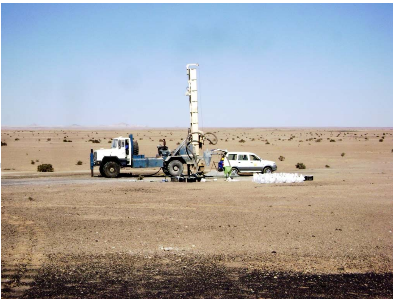
RC Drilling on M1. Note magnetite float in foreground.
