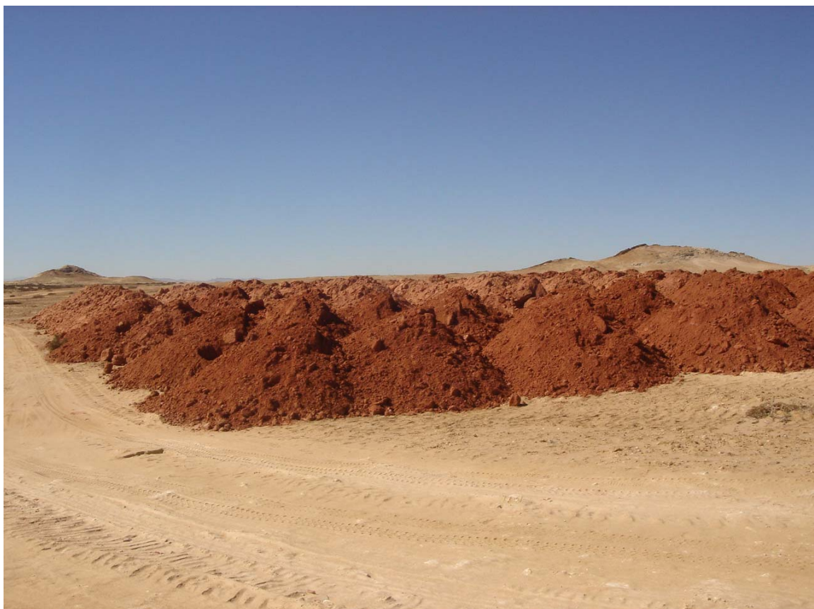
Tubas: Stockpiled mineralised red sand available for testwork
