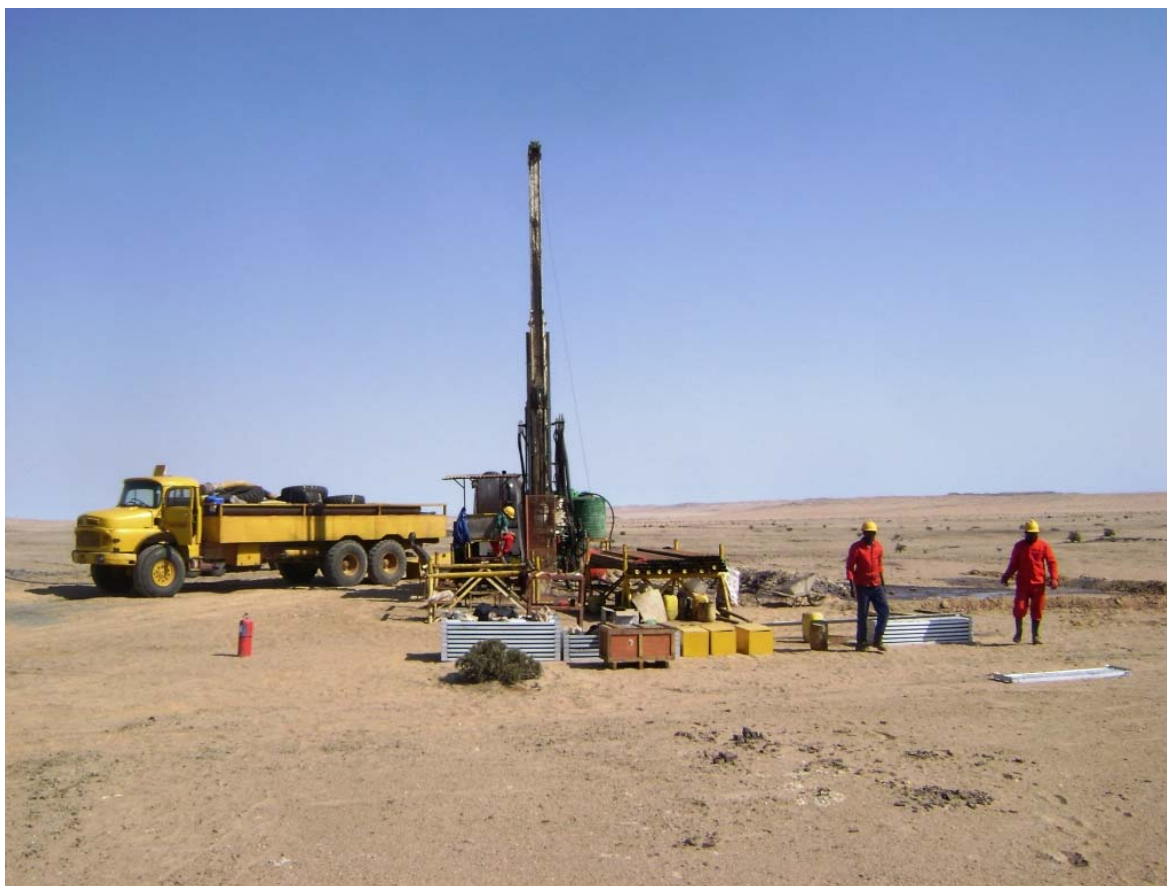
Stratigraphic 500 metre diamond drillhole underway
