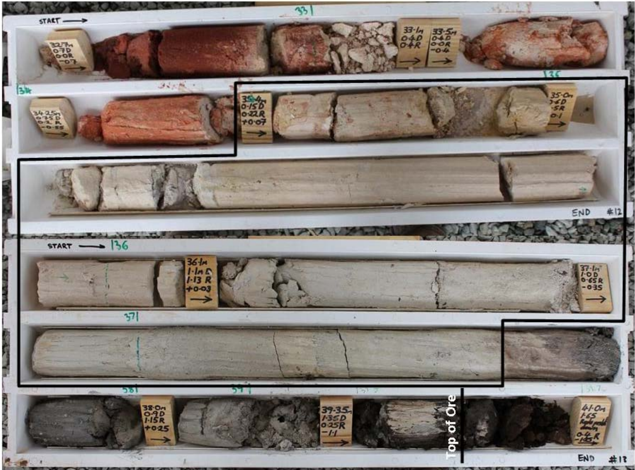
Plate 2.1: Deeper portion of the Oxidised Eocene sediment showing basal kaolinitic clay layer (Black Box) above the orebody at a depth of around 40 m
