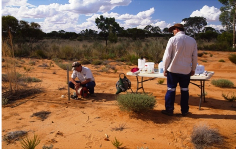
Plate D - 1: Measuring SWL with Heron Water Level Meter
