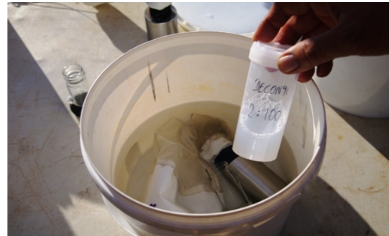
Plate D - 8: Decontaminating Nets Between Holes
