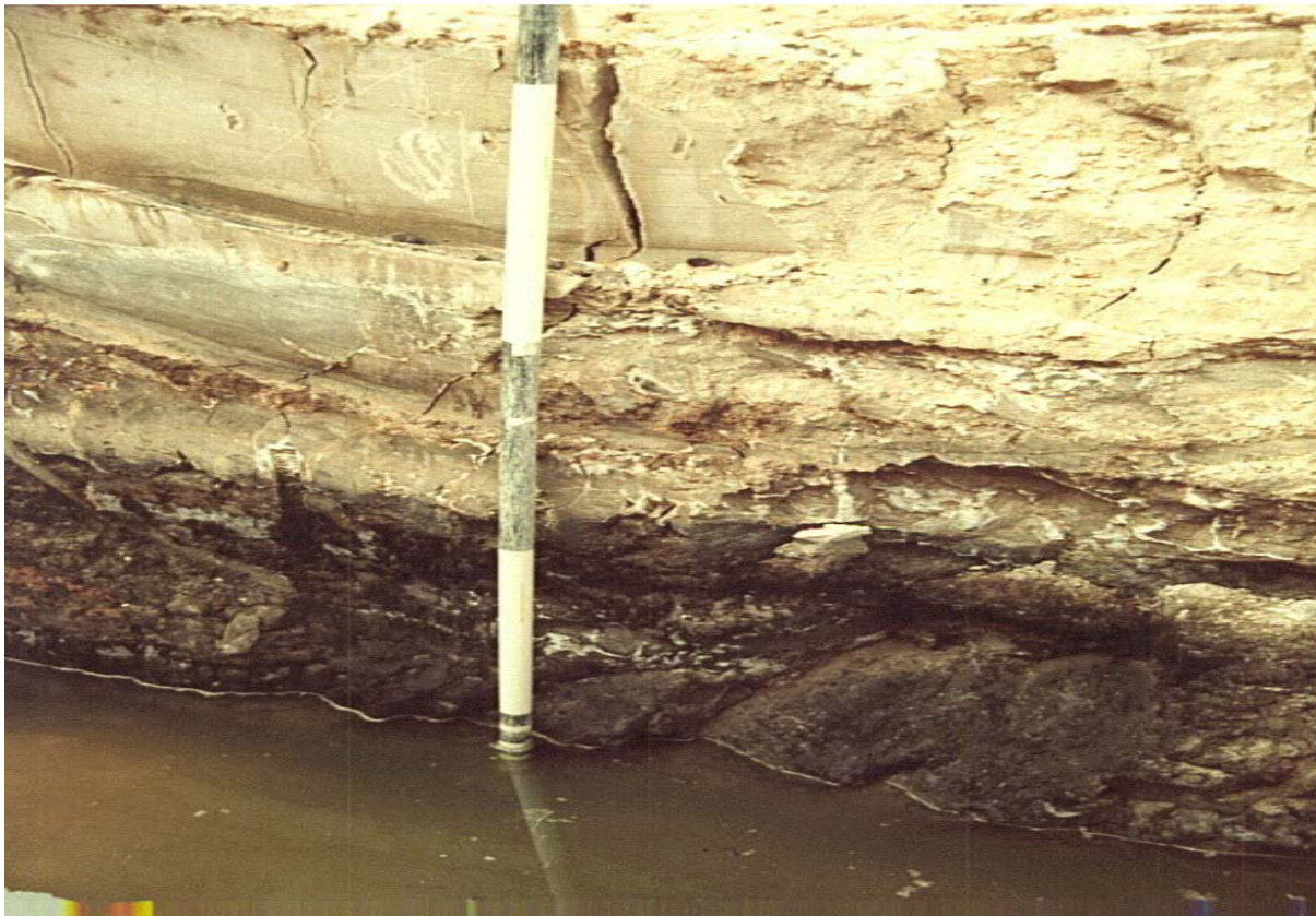
Figure 4 White clay aquitard layer at top of orebody aquifer in PNC trial slot
