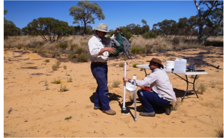
Plate D - 2: Bailing Groundwater Sample
