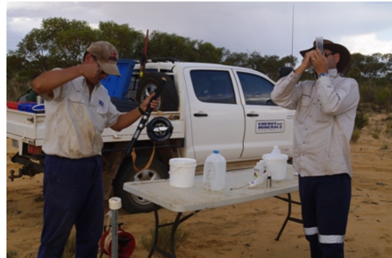
Plate D - 6: Checking Sample Flask Content with Hand Lens
