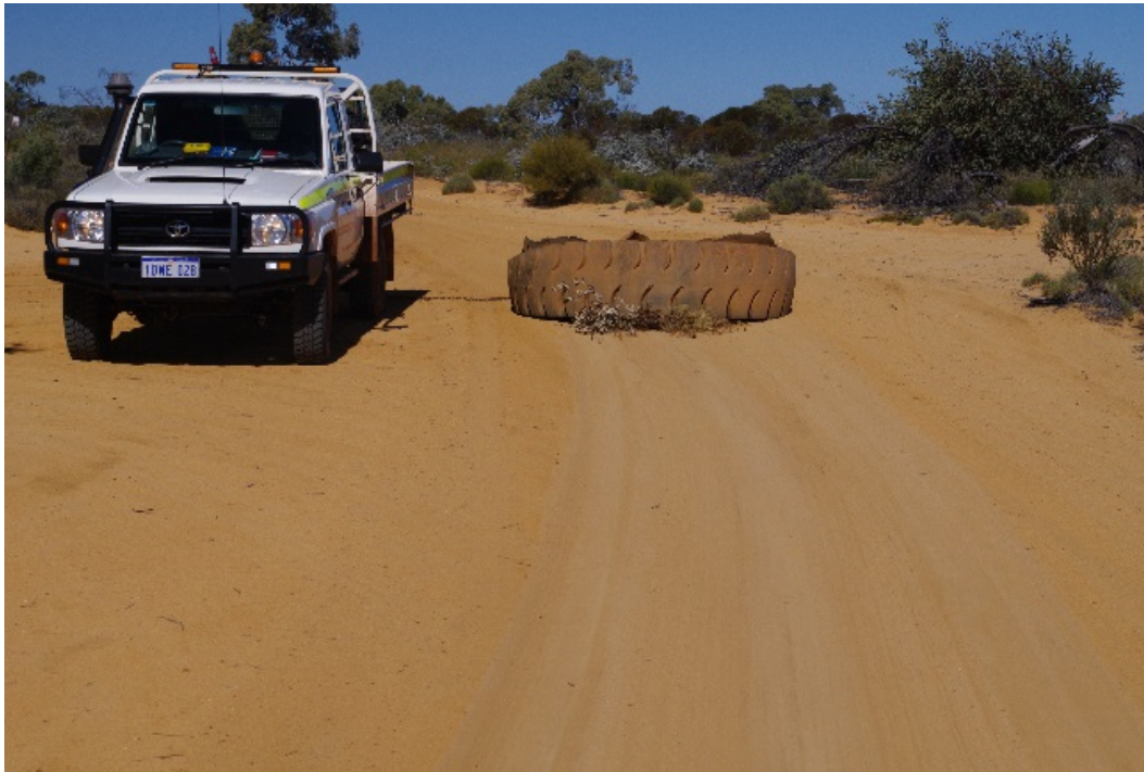
Plate 1: Levelling soft road sand for sand pad monitoring transects
