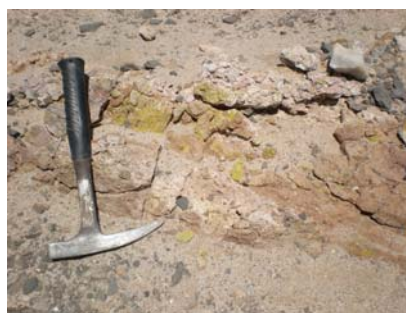
Figure 11: Tumas-3 Palaeochannel Outcropping Carnotite Mineralisation
