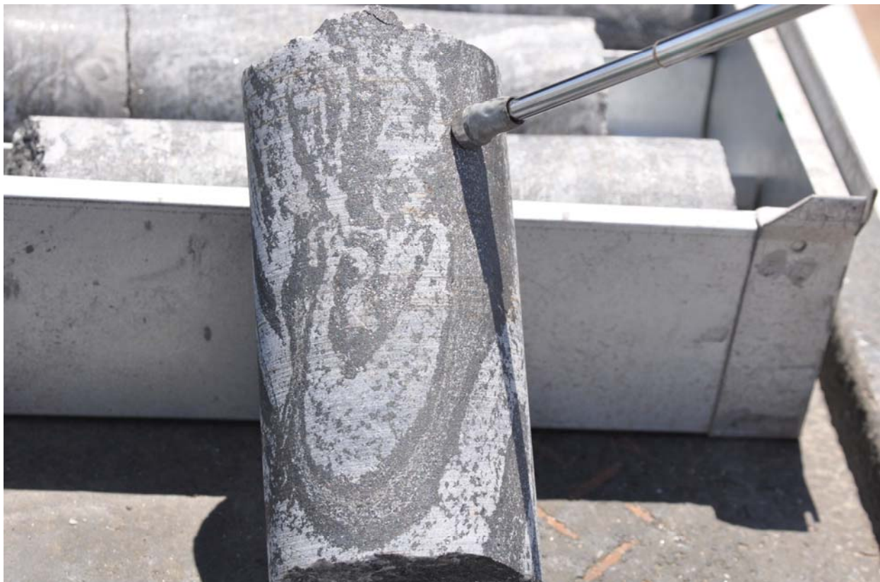
Figure 16: Shiyela PQ Core Showing Folded Magnetite Bands
