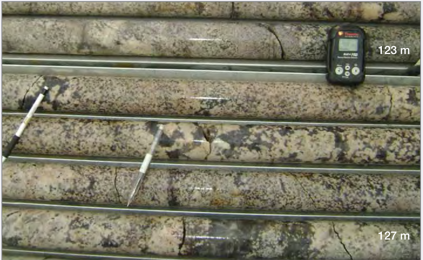
Figure 6: High grade alaskite mineralisation with smoky quartz in diamond hole ALAD001
