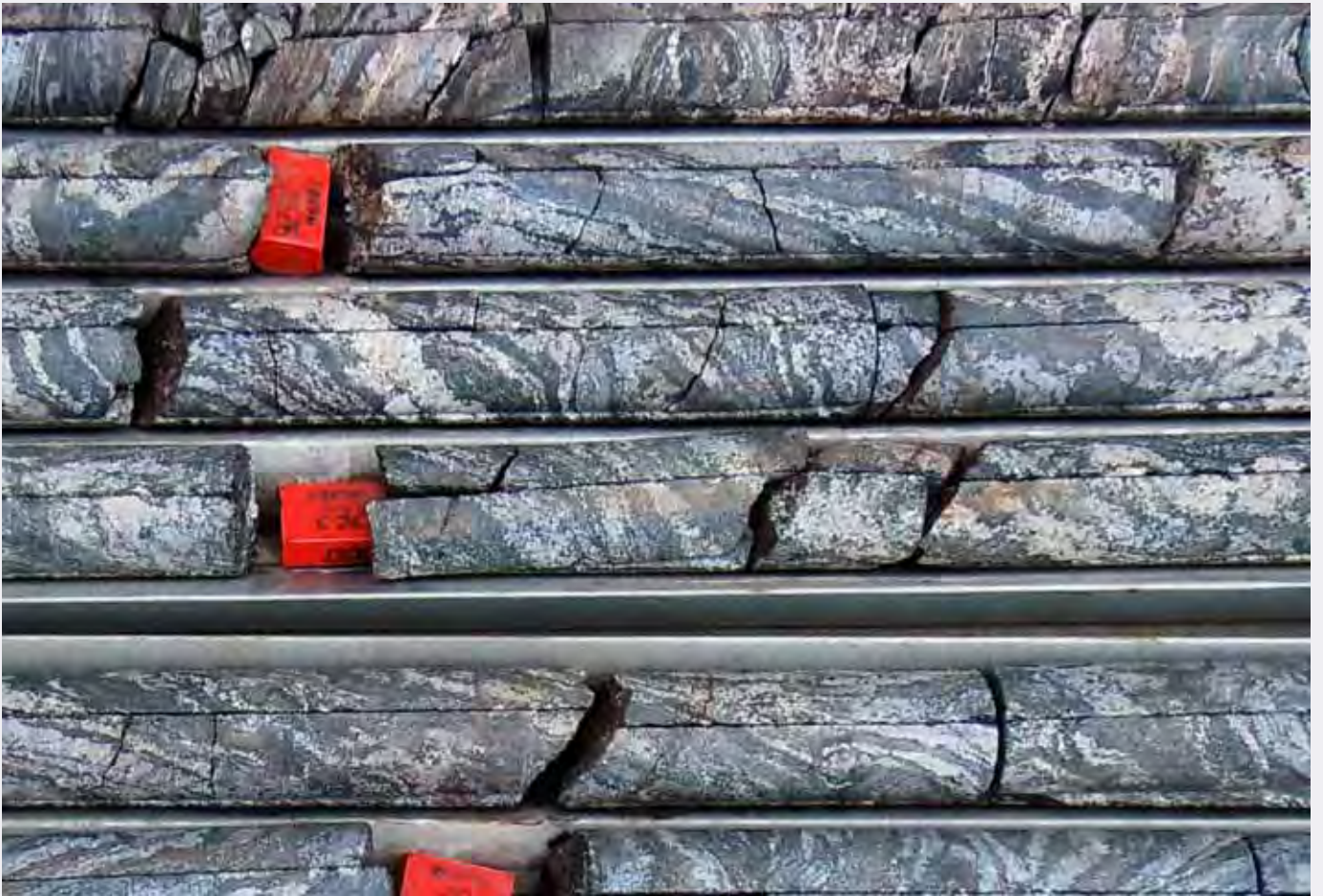
Figure 12: Shiyela Iron Project M63 – Medium to coarse-grained dark grey magnetite bands at 23 metres depth (Hole SHID4)
