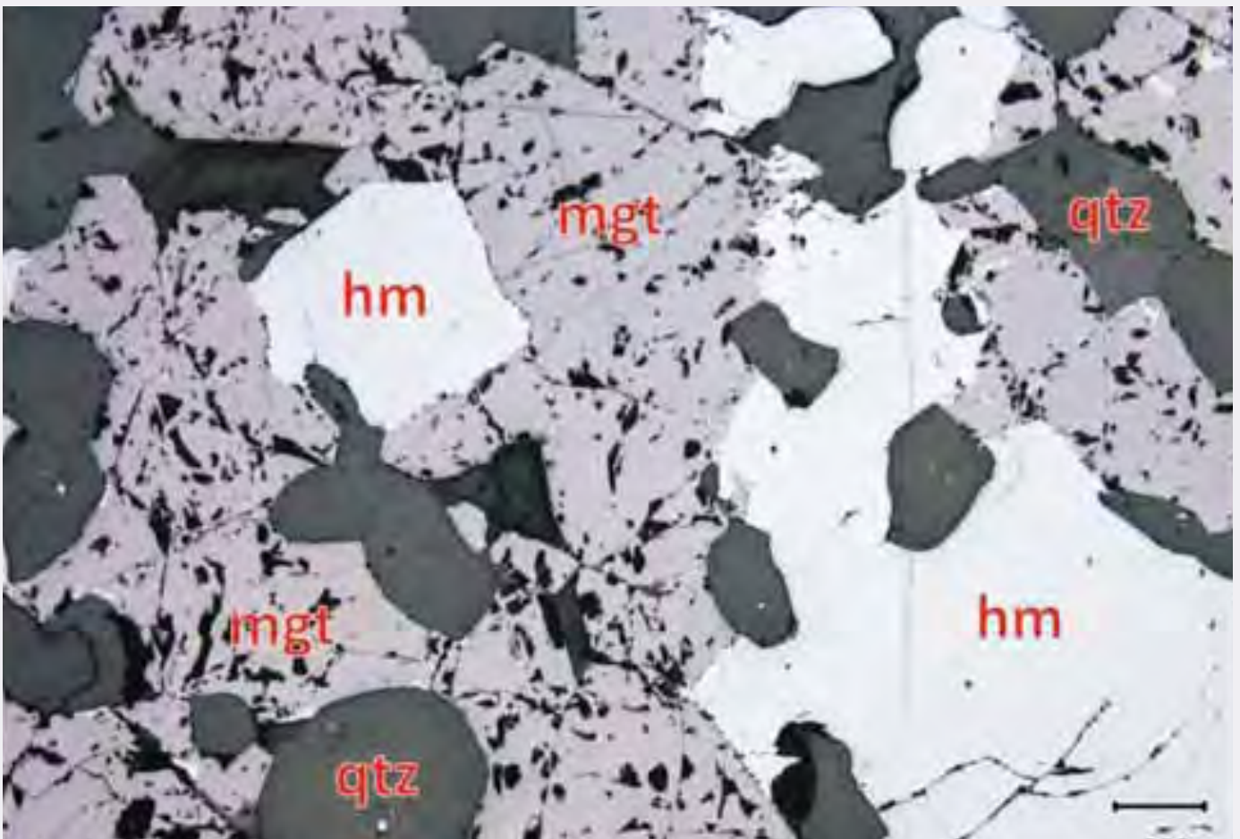
Figure 13: M63: Coarse-grained magnetite (mgt) - hematite (hm) and quartz (qtz)
