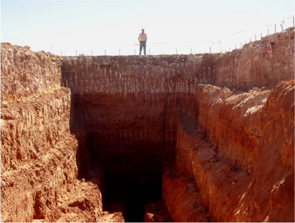
Tubas Trench: Final trench profile showing upper gypsum layer 0 – 2 m depth and mineralised red sand to the bottom of trench
