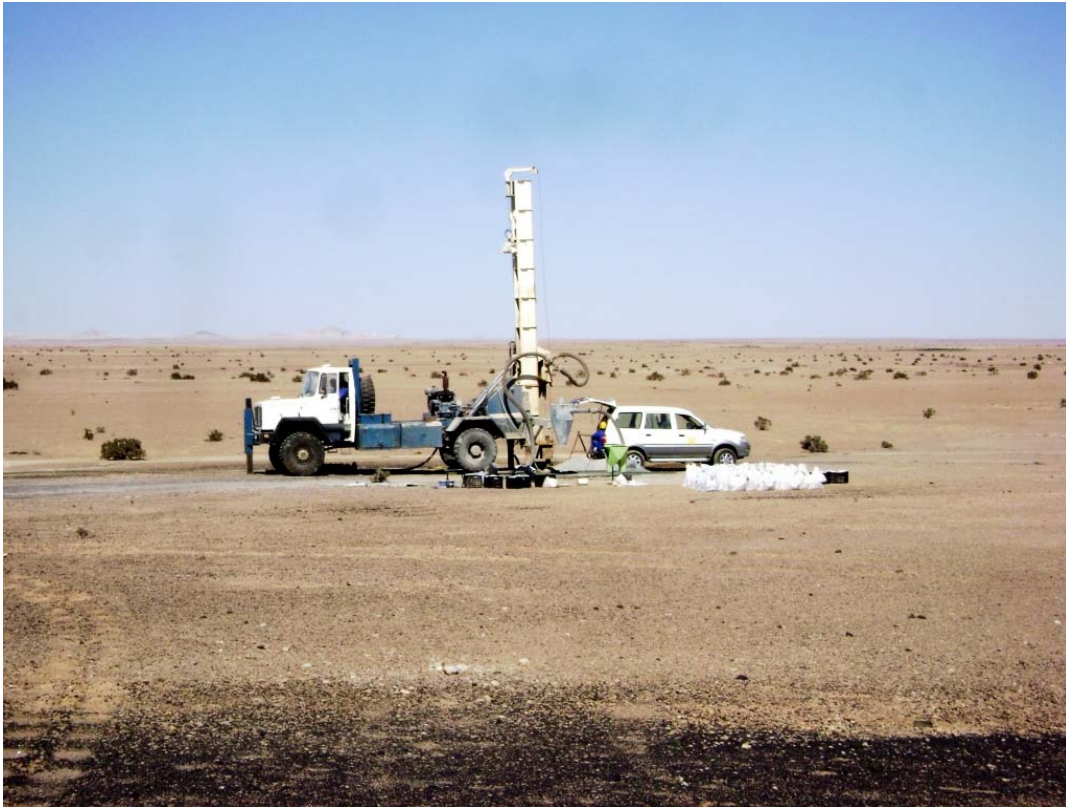
Inca Prospect: RC drilling - note magnetite float in foreground
