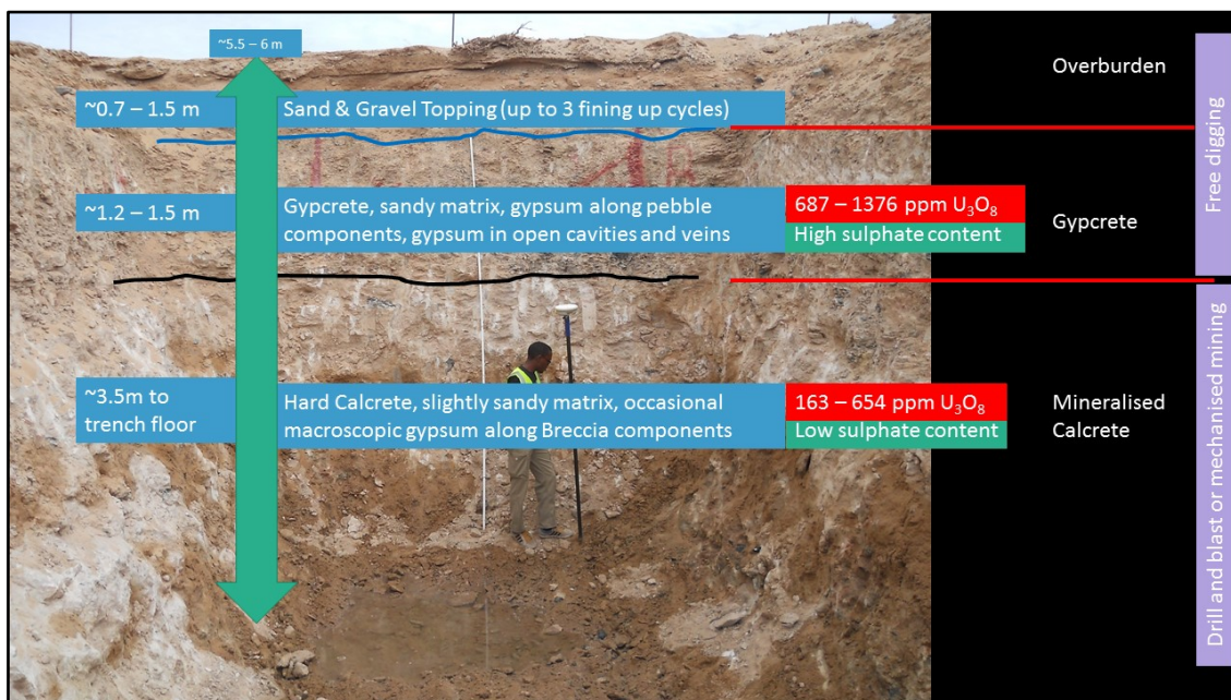
Figure 8: Image of the Tumas Trench showing channel sampling results.
