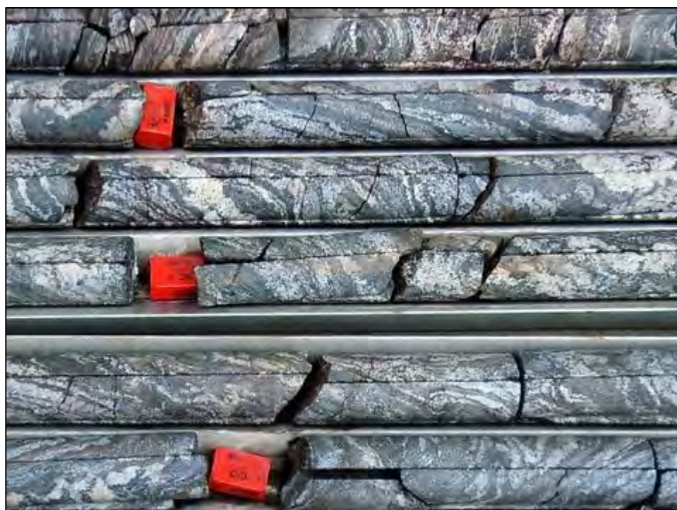
Figure 21 Medium to coarse-grained dark grey magnetite bands at 23 metres depth (Hole SHID4) M63 Deposit
