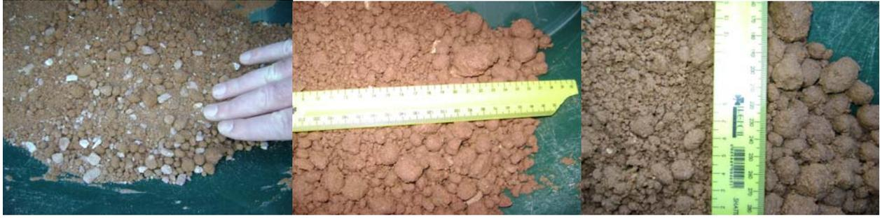
**Figure 6: Progressive formation of agglomerates ending with mechanically hardened agglomerates with and ideal moisture content indicated by a shiny surface.**
