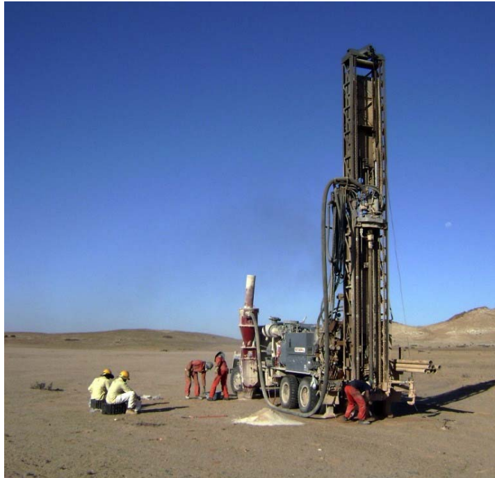
Figure 12: RC Percussion Drilling – Tubas Prospect
