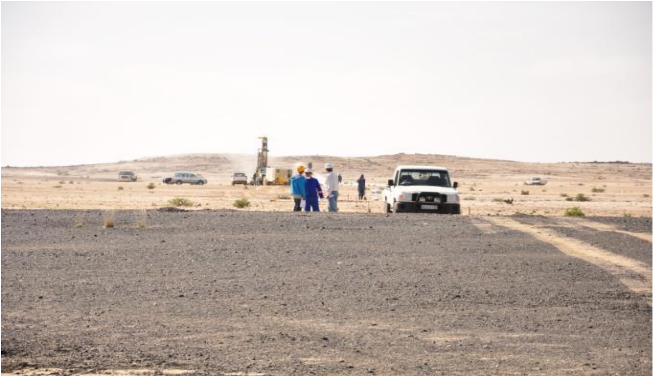
RC Drilling at Ongolo Alaskite Prospect: Foreground is skarn – magnetite subcrop
