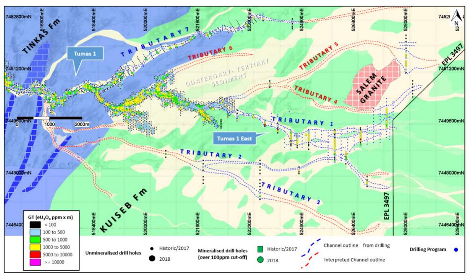
Figure 2: Drill hole locations showing the recent drilling program at Tumas East and Tumas 1. Drill hole collars are coloured in  $eU_3O_8$  grade thickness values (GT:  $eU_3O_8$ pmm x m)
