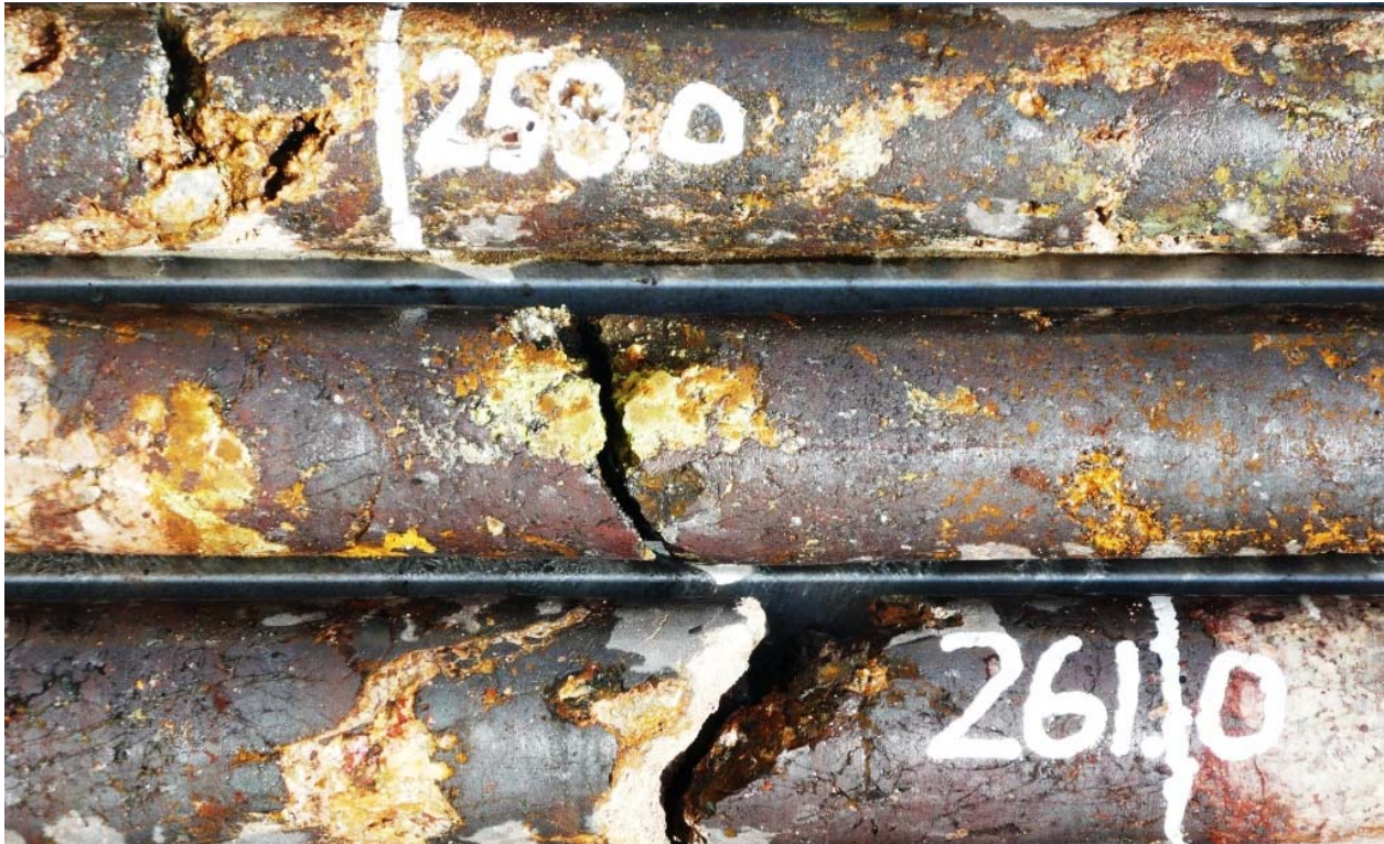
Figure 7: Well-mineralised uraniferous magnetite in HQ diamond core from INCA Deeps
