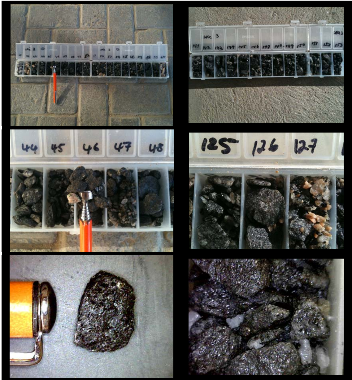
2010 RC drill chips from hole SHIR3 showing zones of semi-massive magnetite
