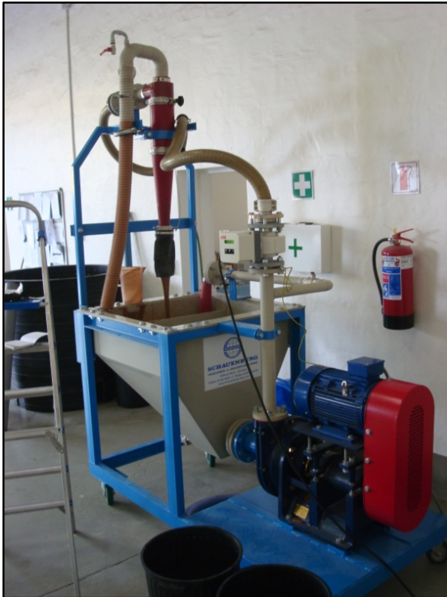
Figure 1. Schauenburg Hydrocyclone Pilot Plant in RUN's laboratory, 2011
