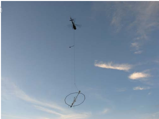
Aeroquest's AEM Helicopter Survey
