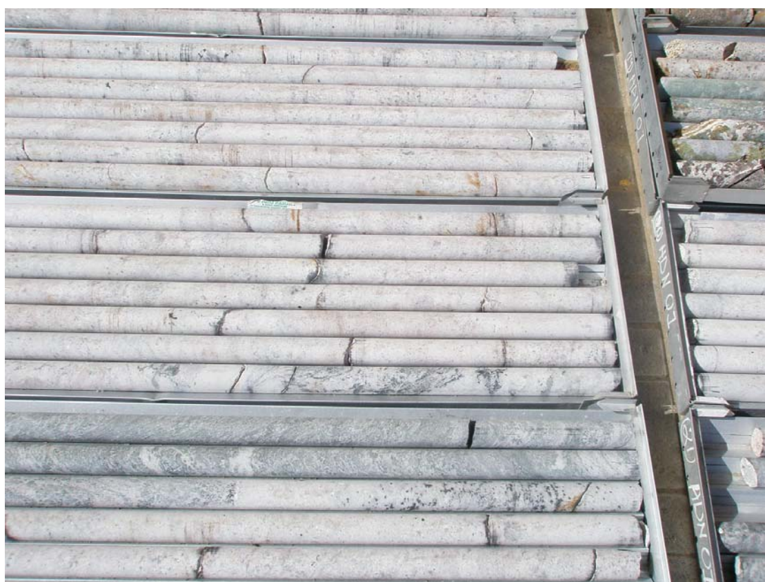
Drill Core Showing White Alaskite (Top Two Trays) and Intercalated Gneissic Granite
