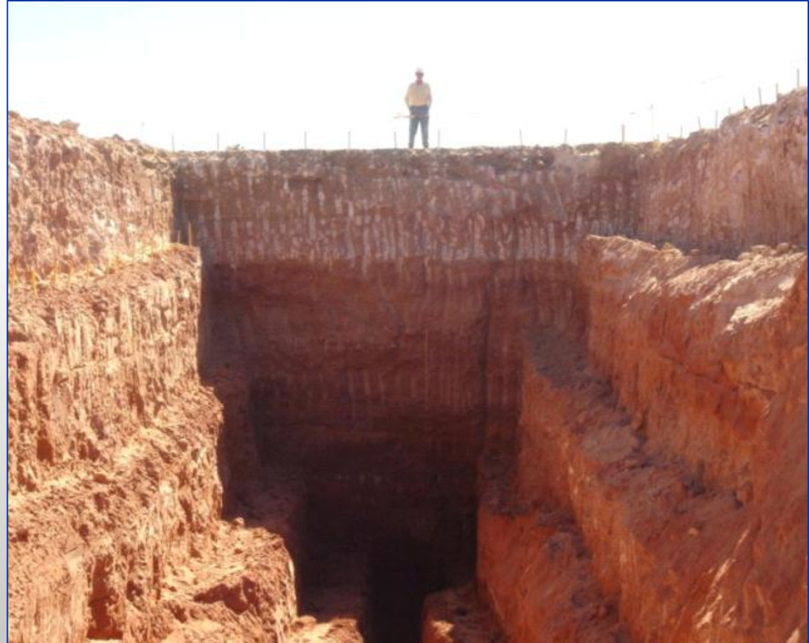
Trench for Bulk Sample
