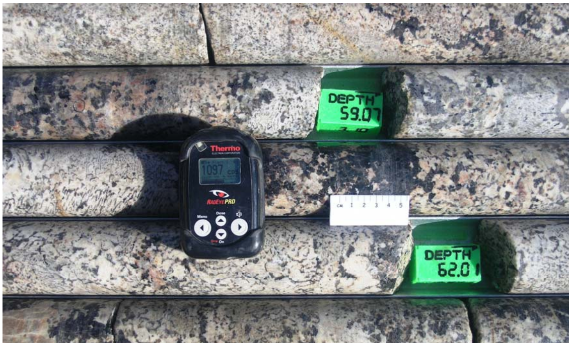
Figure 6: Drillcore ALAD828 - High Grade Mineralisation in Alaskite (white) with Smokey Quartz (dark grey)
