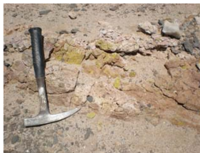
Figure 11: Tumas-3 Palaeochannel Outcropping Carnotite Mineralisation
