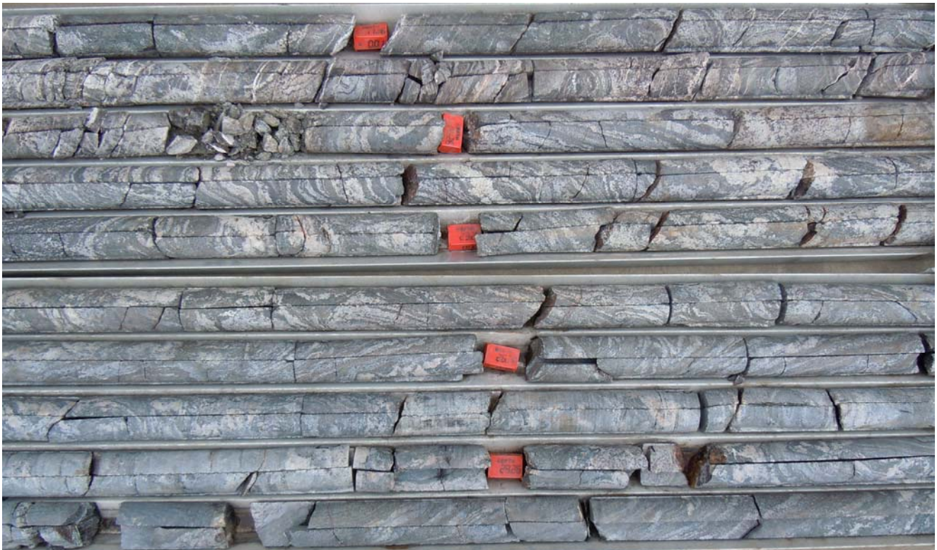
Figure 14: Shiyela Iron Project M63 – Medium to Coarse-Grained Dark Grey Magnetite Bands at 23 Metres Depth (Hole SHID4)
